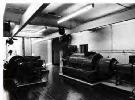
DOWNINGTOWN, PA. — two P-5000 Super-D-Canter centrifuges dewatering co-mixed primary and secondary sludges prior to incineration.
